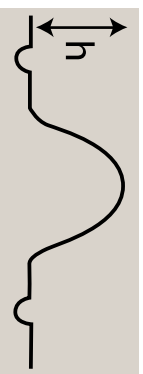
Schema del calcolo dell'indice Erichsen e del LDR (test Swift). Diagram of calculation of Erichsen index and LDR (Swift test).
